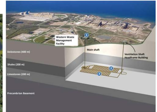
Conceptual design of OPG's Deep Geologic Repository for L/ILW.
